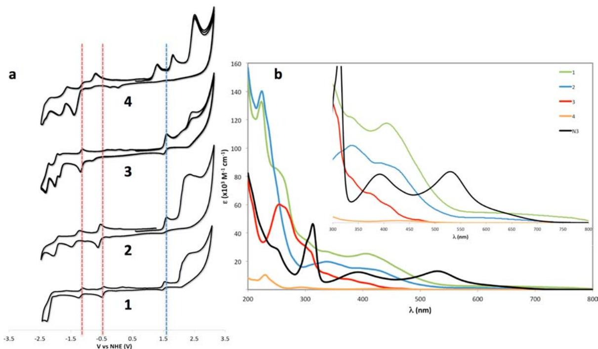
**Figure 2.** (a) Cyclic voltammograms for **1–4** (V vs NHE) recorded at room temperature at 50 mV/s in ACN with 0.1 M  $(\text{tBu}_4\text{N})\text{PF}_6$ . Vertical dotted lines highlight the relative positions of first oxidation and first and second reduction waves with respect to **1**. (b) UV-vis spectra for **1–4** in ACN at 298 K. UV-vis spectrum for N3 in MeOH at 298 K. Inset: Zoomed UV-vis spectra for the low-energy region.
